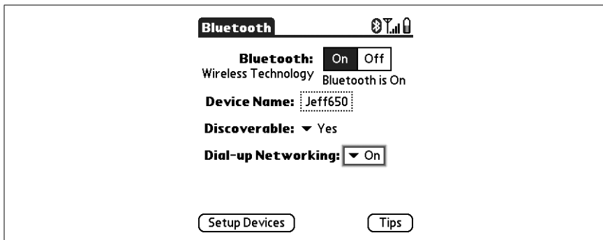
Figure 1-13. Turning on the dial-up networking setting on a Treo 650
